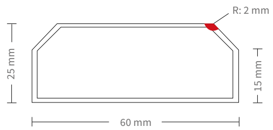
Cross Profile of the Steel Leg (the shell is 1.8mm thick)
